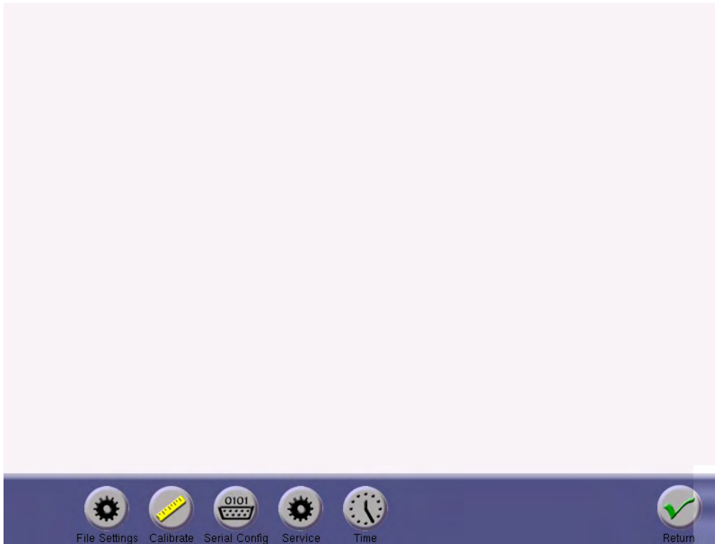
Figure 18: The Setup panel allows the user to configure file settings, calibrate, configure serial output, enter service mode, and configure the instrument time.
