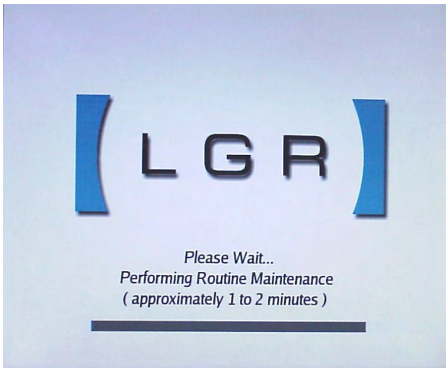
Figure 14: The Routine Maintenance Screen appears during boot-up once a month. Normal operation will automatically continue after the maintenance is complete. Please do not turn off the instrument during maintenance.
