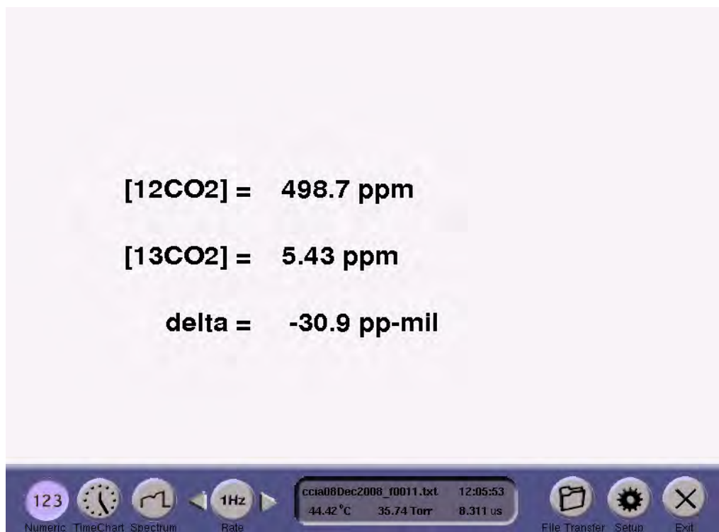
Figure 5: The CO 2 concentration and isotope measurements are reported along with the cell pressure in Torr, cell temperature in Celsius, and the current data filename. The mirror ring-down time in microseconds is measured and reported as well.
