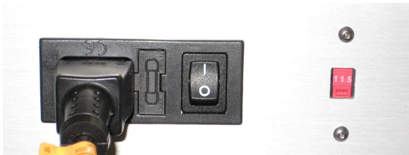
Figure 1: AC power entry module with fuse, power switch, and AC voltage selection switch
