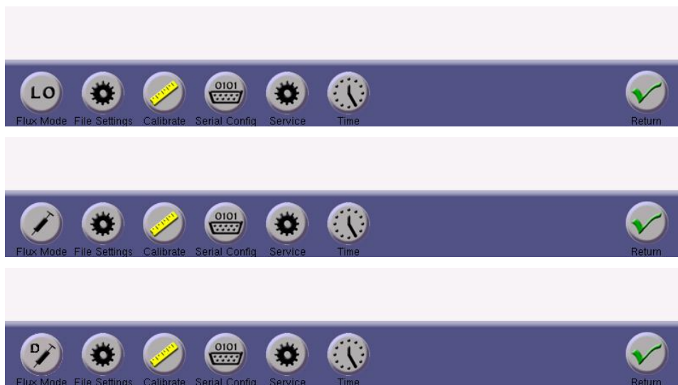
Figure 38: Setup panels displaying various flux modes with the optional batch system installed. Flow through mode (top – LO icon), normal injection (middle – syringe icon), and injection with fixed dilution (bottom – syringe with “D” icon).
