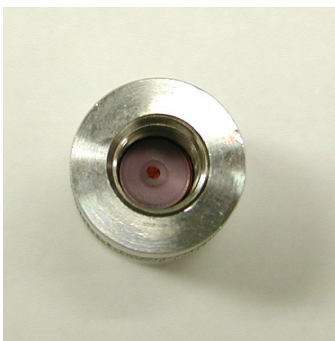
Figure 50: Position of septa within septum nut. Make sure that the Teflon side (white) is facing out.
