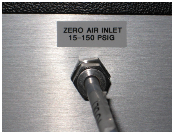
Figure 36: Zero-Air connection port for a \text{CO}_2 Carbon Isotope Analyzer equipped with the optional batch mode system.
