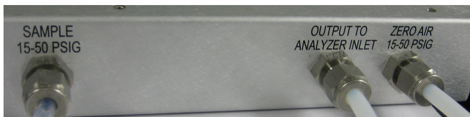
Figure 32: Back panel gas hook-ups for the Dynamic Dilution System (Optional). The sample and the zero-air must be provided with flow capability of 200 sccm and 2.2 slpm respectively.
