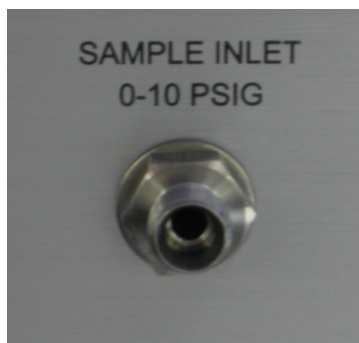
Figure 4: Gas sample inlet connection (1/4"), care must be taken to not over-pressurize.
