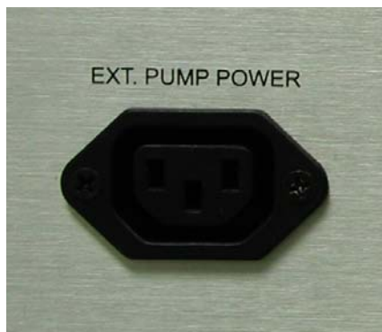
Figure 6: External pump power connection.
