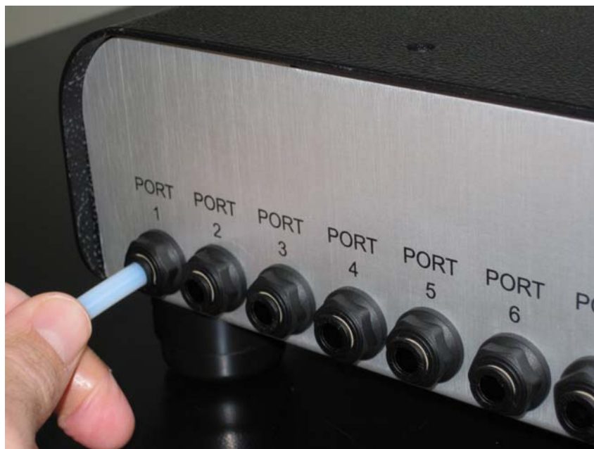
Figure 54: Insertion of sample tube into inlet port '1' on the Multi-port Inlet Unit.,
