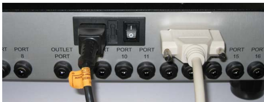
Figure 51: Power and Control connections for the Multi-port Inlet Unit.
