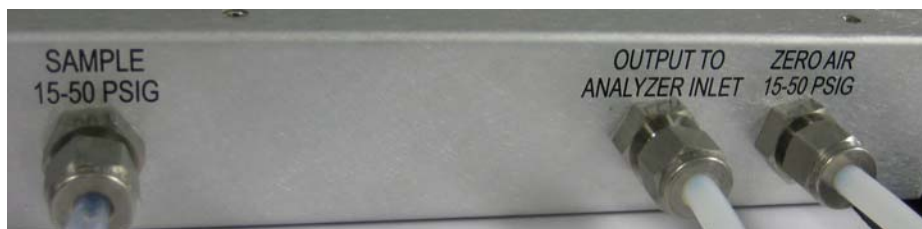
Figure 60: Back panel gas hook-ups for the Dynamic Dilution System (Optional). The sample and the zero-air must be provided with flow capability of 200 sccm and 2.2 slpm respectively.
