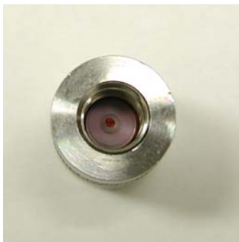
Figure 69: Position of septa within septum nut. Make sure that the Teflon side (white) is facing out.
