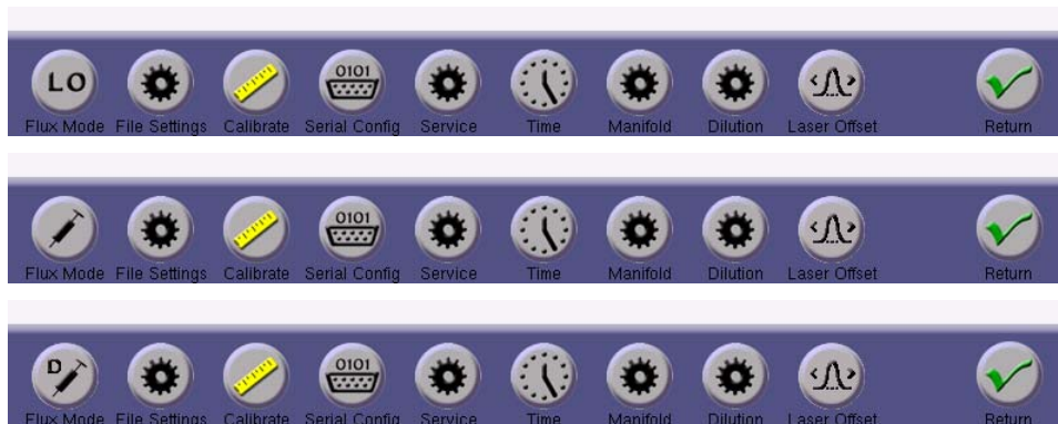
Figure 40: Setup panels displaying various flux modes with the optional batch system installed. Flow through mode (top – LO icon), normal injection (middle – syringe icon), and dilution injection (bottom – syringe with “D” icon).
