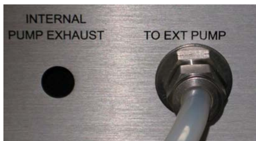
Figure 3: External pump connection (3/8"). The internal pump exhaust port is not used if the instrument has an external pump.
