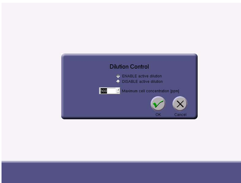
Figure 30: Control Panel for Dynamic Dilution System. If the active dilution is disabled, the control signal remains fixed so that the Dynamic Dilution System has 100% sample flow (no zero-air).
