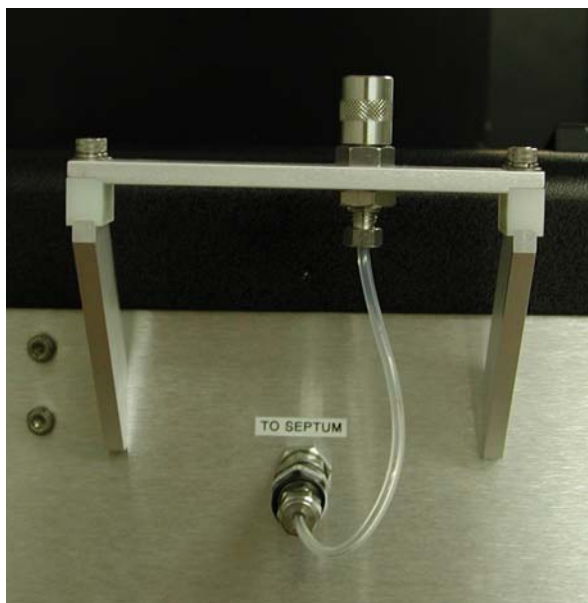
Figure 39: Syringe injection port arm and instrument gas connection for a CO 2 Carbon Isotope Analyzer equipped with the optional batch mode system.
