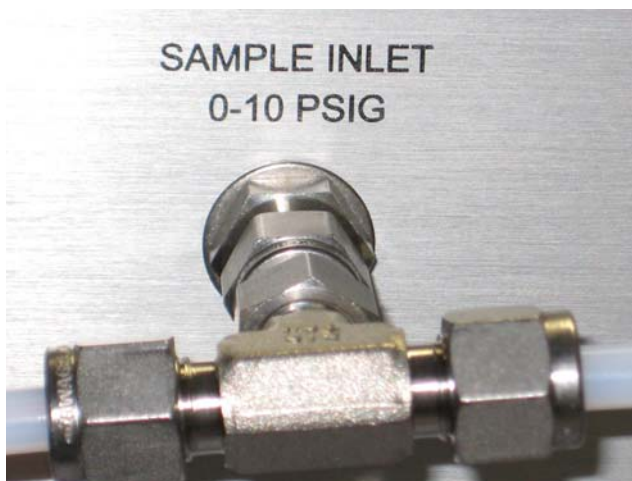
Figure 61: Inlet 'Tee' configuration for Dynamic Dilution System (Optional).
