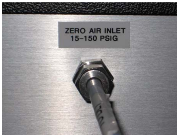
Figure 38: Zero-Air connection port for a CO 2 Carbon Isotope Analyzer equipped with the optional batch mode system.
