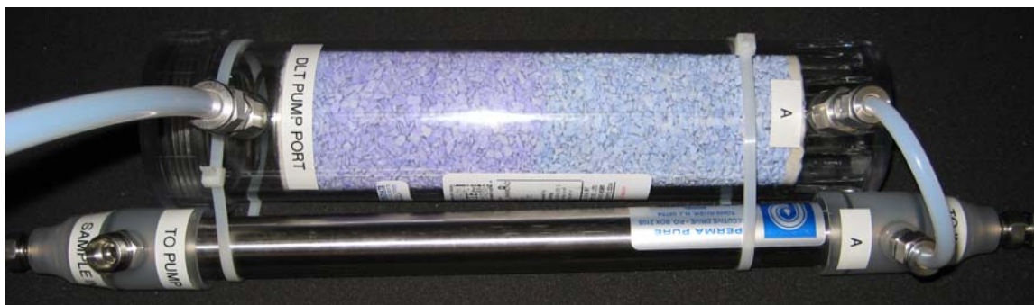
Figure 66: Nafion and Drierite filters for drying gas sample.
