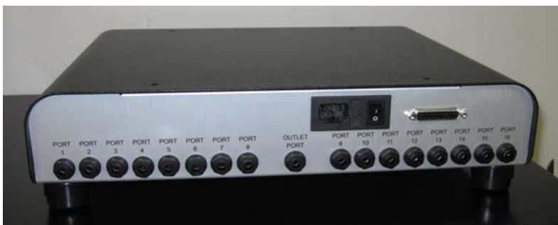
Figure 50: Multi-port Inlet Unit (back view) showing the various connections. The unit supports up to 16 inlet ports labeled numerically. The outlet port connects to the CO 2 Carbon Isotope Analyzer gas inlet. The included 25-pin control cable connects the instrument to the Multi-port Inlet Unit. An additional power cable is included to power the Inlet Unit.
