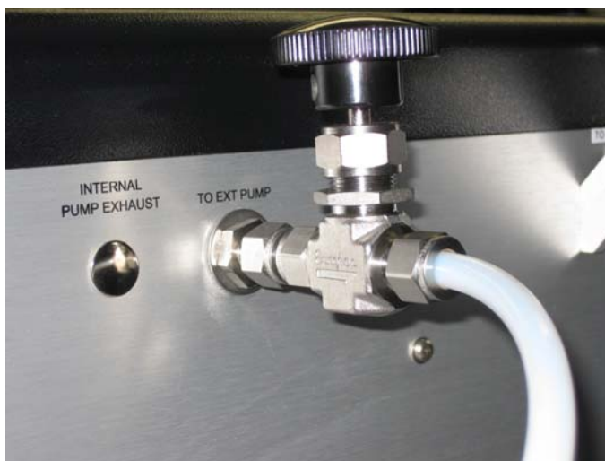
Figure 62: Optionally provided throttle valve for trimming instrument flow to less than 180 sccm for proper Dynamic Dilution control. This valve is only provided (externally) if the user needs to adjust instrument flow to go between Dynamic Dilution and Batch Mode Operation.
