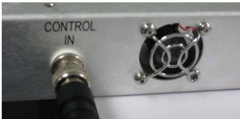
Figure 63: “Control In” connection on the Dynamic Dilution System.
