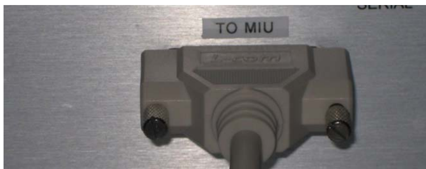
Figure 52: Connection of Multi-port Inlet Unit control cable to back of CO 2 Carbon Isotope Analyzer.
