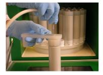
Remove the reference vessel from the shields
