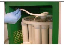
WARNING: Touch only the metal connector. As shown in the previous picture, it is important to handle the sensor only through the connector. This will avoid any possible damage of the sensor.
