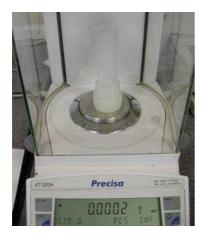
Tare the vessel and directly weigh the sample by placing it inside the vessel.
