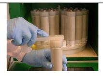
Introduce the ATC-400 sensor (050214/M6) into the thermowell (MUR00011/M6)
