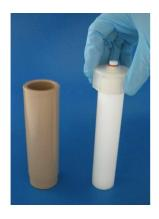
Un-tight and remove the cover and rinse it using distilled water
