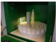
Introduce all the standard vessels into the rotor.
