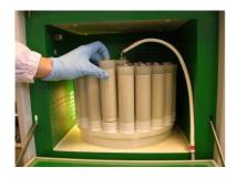
Remove the TFM vessel from the safety shield
