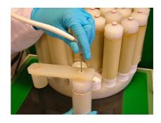
...and tight the PTFE adapter of the sensor into the thermowell
