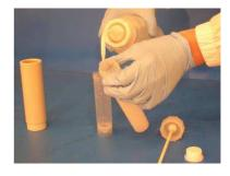
Transfer the digested solution into a suitable volumetric flask
