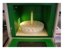
Introduce a standard vessel into the rotor body
