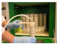
Remove the sensor by losing the threaded adapter and the reference holder
