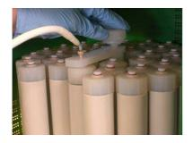
Place the ring cover on the rotor. The sensor must pass trough the ring.
