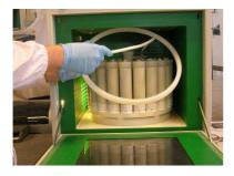
Plug in the ATC-400 Temperature sensor to the device control of the Microwave unit.
