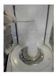
Add suitable reagents to the sample. When part of the sample is left on inner wall of the vessel, try to wet it by adding acids drop by drop. Gently swirl the solution, to homogenize the sample with the reagents.
