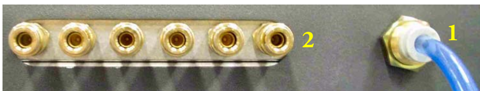
Figure 2-48. Compressed Air Inlet and Compressed Air Connections
