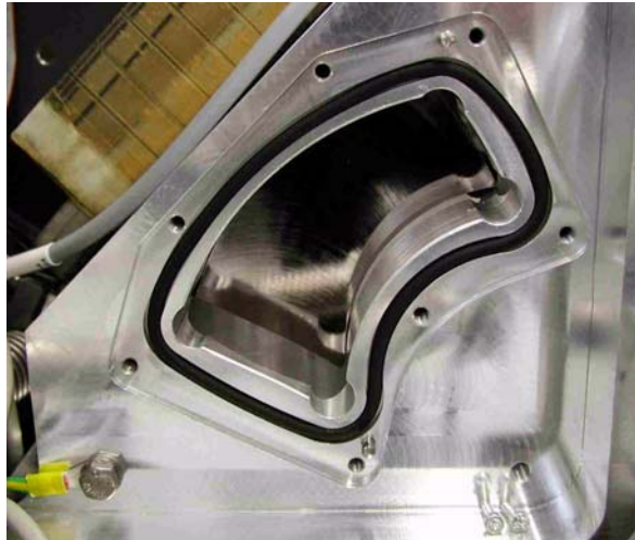
Figure 5-20. View into Analyzer - One Magnetic Coil Dismantled
