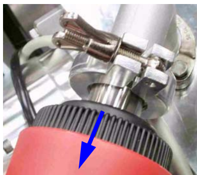
Figure 7-27. Pulling Away Electronics Cylinder of Penning Gauge
