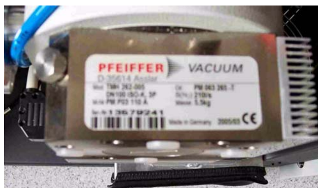
Figure 7-15. Heat Sinks Mounted upon Analyzer Turbo Pumps
