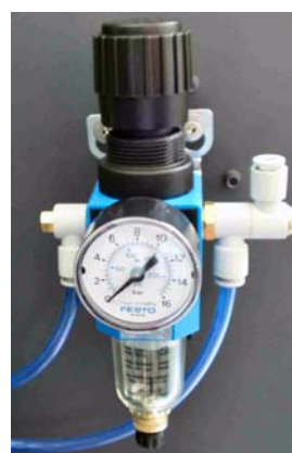
Figure 2-30. Pressure Reducer for Compressed Air - Front View
