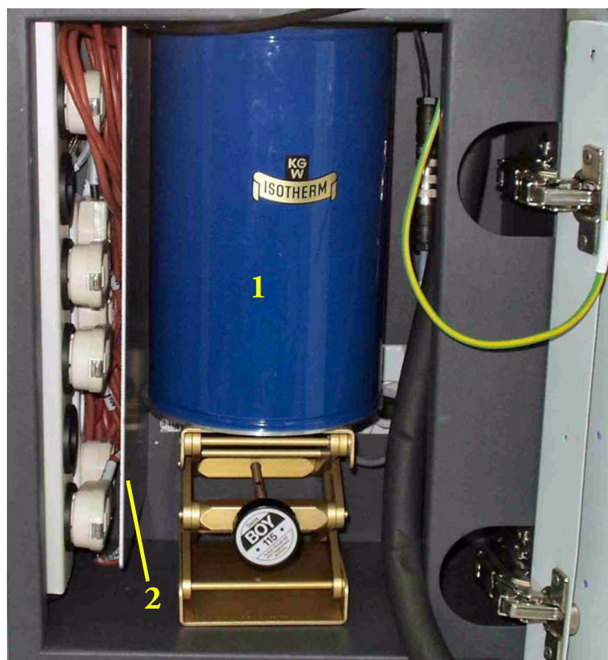
Figure 2-18. Position of Microvolume within Microvolume Cabinet
