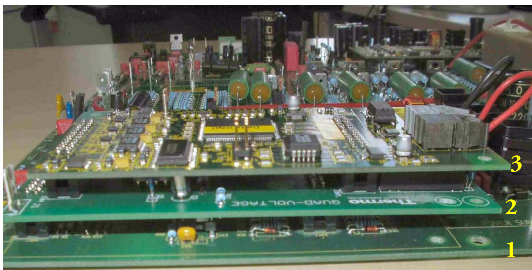
Figure 2-61. Arrangement of Focus Quad Power Supply Board
