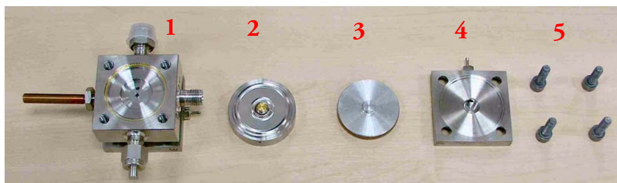
Figure 4-4. Parts of Dual Inlet System Valve
