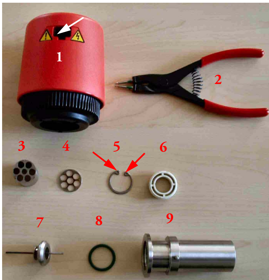
Figure 7-29. Dismantled Parts of Penning Gauge
