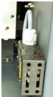
Figure 2-12. Safety Contact for Door
