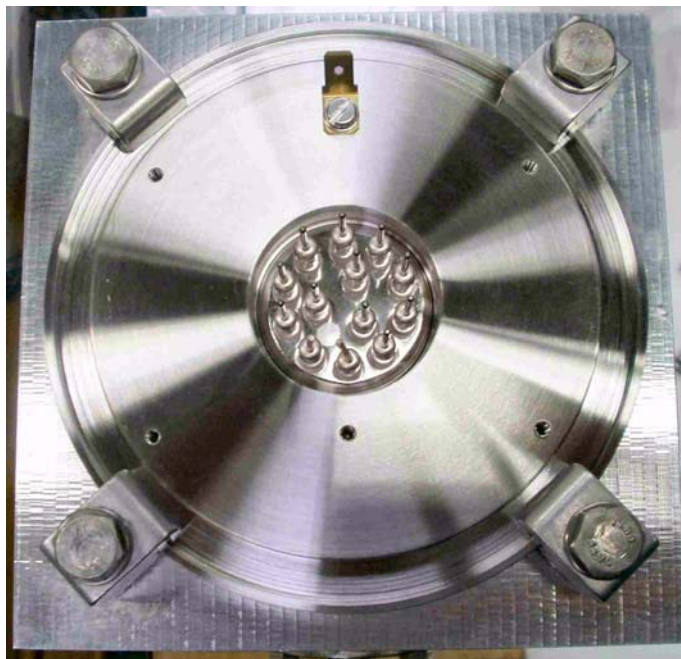
Figure 7-6. Ion Source Flange
