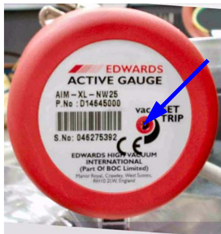
Figure 2-41. Penning Gauge - Implemented (Front View)
