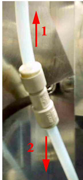
Figure 2-38. Check Valve Near Three-Way Valve
